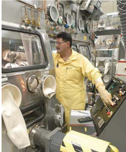
Figure D-10. A machinist operates a precision lathe inside a glovebox.
